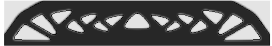
(a) V/V_0 = 0.7 (°/1); Compliance = 1.726 \cdot 10^2 N·mm
