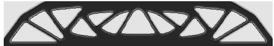
(c) V/V_0 = 0.5 (°/1); Compliance = 2.151 \cdot 10^2 N·mm
