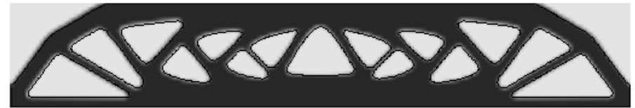
(b) V/V_0 = 0.6 (°/1); Compliance = 1.893 \cdot 10^2 N·mm
